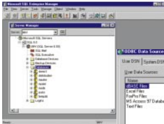
Fig 10 (right) Using the DSA to create an ODBC data source, in this case a user-specific one
